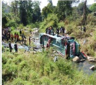
Figure 2 – Bus rolled with its right side on ground. The roof, upper floor passenger cabin and all seats were thrown away during rollover.
